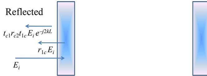
$$\begin{aligned} \frac{E_{\text{reflected}}}{E_i} &= r_{1c} + t_{c1} r_{c2} t_{1c} e^{-2jkL} + t_{c1} r_{c2} r_{c1} r_{c2} t_{1c} e^{-4jkL} + \dots \\ &= r_{1c} + \frac{t_{c1} r_{c2} t_{1c} e^{-2jkL}}{1 - r_{c1} r_{c2} e^{-2jkL}} \end{aligned}$$
