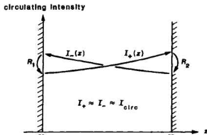
*The interference between the right- and left-traveling waves is neglected.*
