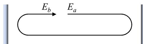
The noise radiation originated from the spontaneous emission exponentially grows and leads to a coherent self-sustained oscillation inside the cavity if net gain is greater than the net loss.
